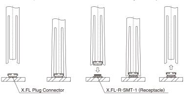
(2) Allowable load to a cable that is mated
