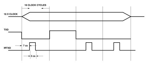
The encoder sends a pulse for every space or "0" that is sent on the TXD line. On a high to low transition of the TXD line, the generation of the pulse is delayed
