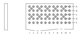
Recommended PCB hole mounting pattern for row differential applications. (Same geometry as above without the ground vias.)
