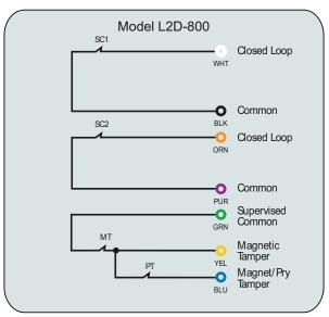
All Circuits Shown with Magnet Actuator in Secure Position. For Built-in EOL Resistor Configurations and Values (not shown), Visit WWW.MAGNASPHERE.COM.
