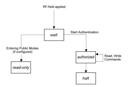
After entering the RF-field the transponder waits for a command to start the authentication.
