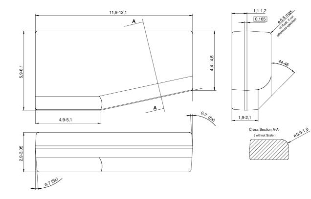
Protruding plastic must not exceed specified dimension by more than 0.2 mm
