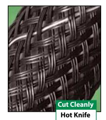
HALAR® (HT) self-extinguishing sleeving is used where flammability, high temperature endurance and low outgassing are primary concerns. HT is braided from 11 mil ethylene chlorotriflouroethylene (ECTFE) copolymer monofilament.
