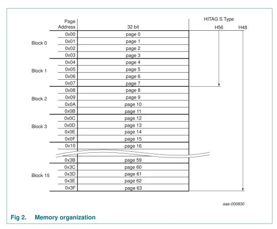
The EEPROM has a capacity up to 2048 bit and is organized in 16 Blocks, consisting of 4 Pages each, for commands with Block access. A Page consists of 4 Bytes each (1 Page = 32 Bits) and is the smallest access unit.
