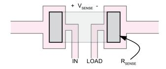
Choose a low inductance type sense resistor if preservation of bandwidth is important. The use of Kelvin connections helps by excluding the inductive voltage drop across the traces leading to the sense resistor. The inductive voltage drop may be substantial when operating at high frequencies.
