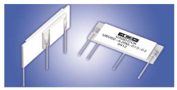
**Type USVD Ultra-Precision Voltage Dividers** have the very highest precision available in voltage dividers in the range of 450 Volts DC up to 2000 Volts DC. These dividers are formed by bonding together two selected Type USF Ultra-Precision Resistors. The precise selection of these high performance resistors, which form the voltage dividers, makes possible the outstanding voltage division performance. Ratio Tolerance as tight as 0.01% and Ratio TC of 2ppm/°C.
