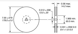
Standard Qty/Reel is 1000; maximum available quantity per reel is 3,500 for 1206 size and 2,000 for 2512 size; call 1-866-9-OHMITE for details.
