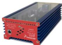
The Freescale High-Voltage Development Platform is a set of software and hardware tools for evaluation and development of high-voltage motor control and power conversion algorithms. It is ideal for rapid prototyping of high-voltage microcontroller-based applications.
