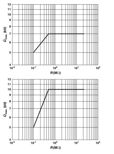
$\label{eq:main_state} \begin{aligned} & \textbf{HVR25} \\ \Delta R = \pm \; (4.0 \; \% \; R + 0.1 \; \Omega) \end{aligned}$
