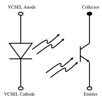
It is recommended in application that a  $100-1000\Omega$ load resistor be connected between the emitter and a negative power supply between 5 and 15V. The output can be read as the voltage across the resistor. Alternatively, the case can be connected to a power supply with the load resistor remaining connected to the emitter.
