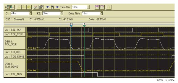
Figure 20: TDO\_DONE\_MISO Timing with Respect to TCK\_CCLK\_SCK (TCK\_CCLK\_SCK to TDO\_DONE\_MISO Delay)
