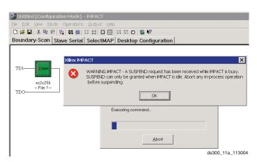
Figure 12: Suspend Warning When iMPACT Is Busy
