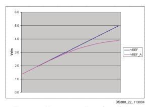
Figure 23: V<sub>REF A</sub> as a Function of V<sub>REF</sub>
