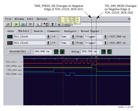
Figure 18: TDI DIN MOSI and TMS PROG SS Timing with Respect to TCK CCLK SCK
