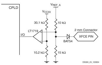
Figure 24: Target Interface Receiver Topology
