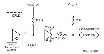
Figure 22: Target Interface Driver Topology
