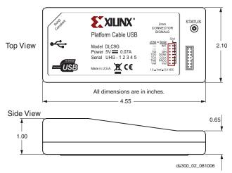
Figure 2: Plastic Case Physical Dimensions
