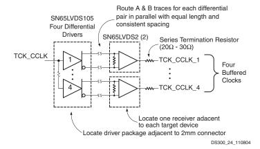
Figure 25: Differential Clock Buffer Example
