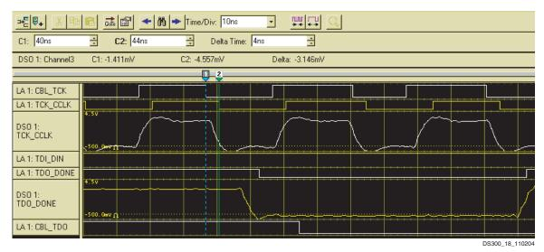
Figure 19: TDO\_DONE\_MISO Timing with Respect to TCK\_CCLK\_SCK (CBL\_TCK to TCK\_CCLK\_SCK Delay)
