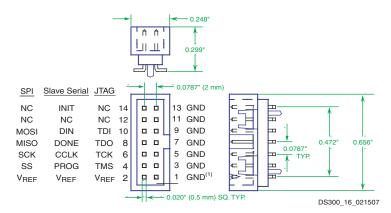
Figure 17: Target Interface Connector Dimensions and Signal Assignments
