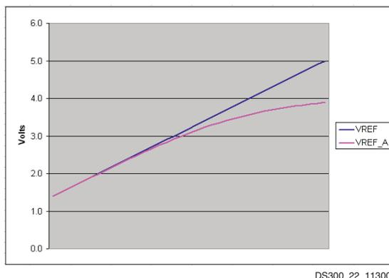
Figure 23:  $V_{REF\_A}$  as a Function of  $V_{REF}$
