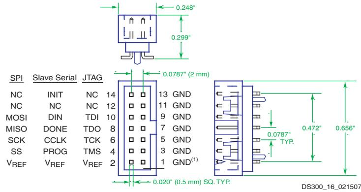
Figure 17: Target Interface Connector Dimensions and Signal Assignments
