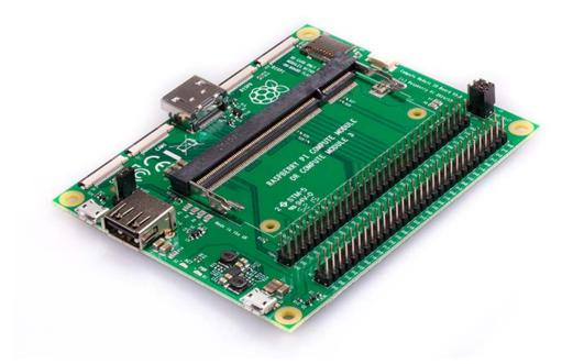
The Compute Module IO Board V3 is a development kit for those who wish to make use of the Raspberry Pi in a more flexible form factor, intended for industrial applications. The IO Board V3 is made for developing with CM3, CM3L, and CM1. This kit replaced the original Compute Module IO Board in January 2017.
