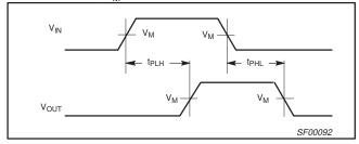
Waveform 1. Propagation Delay for Non-Inverting Outputs
