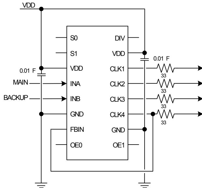
In this example, the clocks are 155 MHz and so the frequency range is address 11. Both S0 and S1 are left unconnected, causing the on-chip pull-ups to produce the required high inputs. The same is true for OE0, OE1, and DIV. In this example, CLK4 is used as the feedback. Note that the feedback path is before the series resistor.
