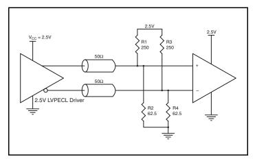
Figure 4A. 2.5V LVPECL Driver Termination Example
