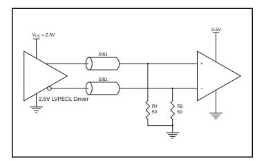
Figure 4C. 2.5V LVPECL Driver Termination Example
