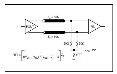
Figure 3A. 3.3V LVPECL Output Termination
