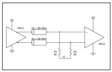
Figure 5A. 5V LVPECL Driver Termination Example
