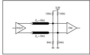
Figure 3B. 3.3V LVPECL Output Termination
