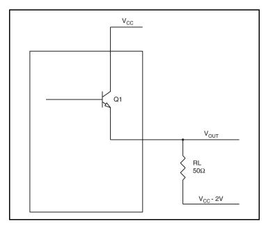
Figure 6. LVPECL Driver Circuit and Termination
