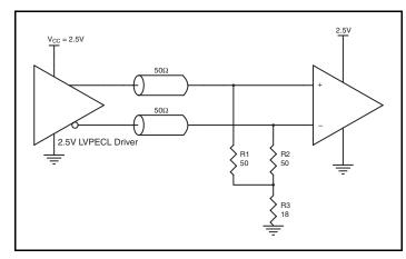
Figure 4B. 2.5V LVPECL Driver Termination Example
