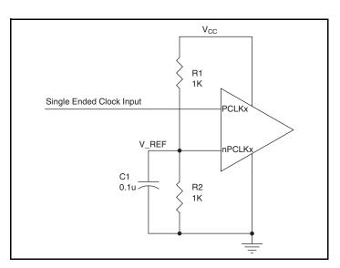
Figure 1. Single-Ended LVCMOS Signal Driving Differential Input
