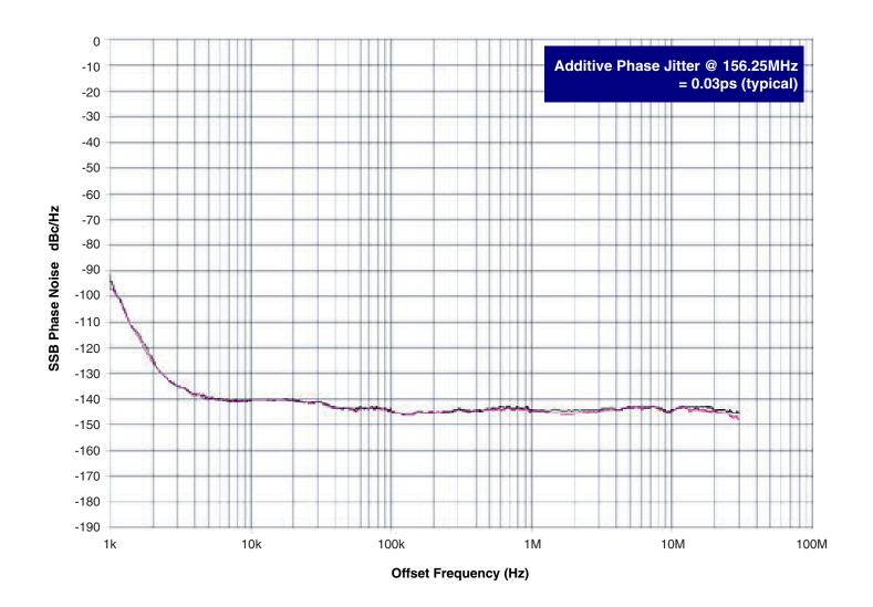
As with most timing specifications, phase noise measurements has issues relating to the limitations of the equipment. Often the noise floor of the equipment is higher than the noise floor of the device. This is illustrated above. The device meets the noise floor
