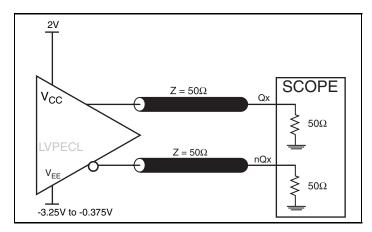
**LVPECL Output Load AC Test Circuit**
