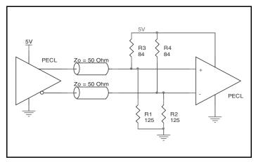
Figure 5B. 5V LVPECL Driver Termination Example
