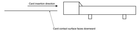
2. After the smart card has been inserted, be sure not to appy excessive force to the card portion that protrudes from the insertion slot.
