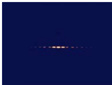
Figure 6. Laser diffraction pattern from dual slit.
