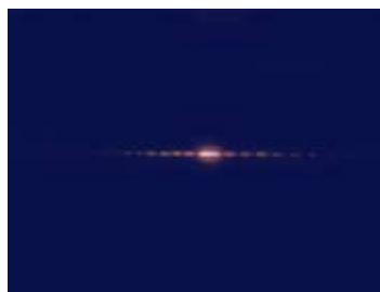
Figure 5. Diffraction pattern created by two razor blades.
