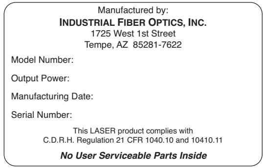
Figure 3. Laser certification and identification label.
