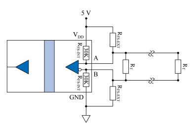
resistors and up to four RS-485 worst-case Unit Loads of 12 k $\Omega$ .
