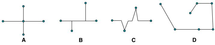
Configurations A and B have long spurs that can cause reflections. Short spurs from the bus to intermediate nodes are generally necessary, however. If so, stub lengths should be less than one-sixth the electrical signal length, which is defined as:
