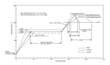
Recommended profile shown. Maximum temperature allowed on any profile is 260° C.
