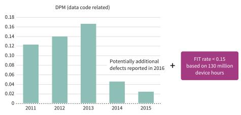
CoolMOS<sup>™</sup> comes with a DPM of less than 0.1 and FIT rate of less than 0.15
