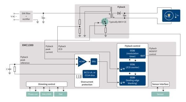
AC/DC application example 2: 2-channel flyback PFC constant current LED driver with DALI, 0–10 V and phase-cut dimming option
