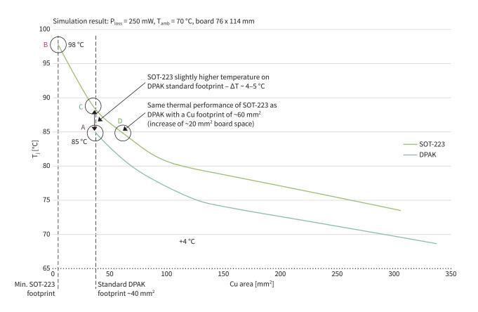
The laboratory findings on thermal behavior are confirmed by a thermal simulation with  $T_{ambient} = 70$  °C and  $P_{loss} = 250$  mW. The size of the copper area in the footprint is shown on the x-axis, while the y-axis displays the temperature of the package top side. In the case of an SOT-223 on DPAK footprint, the 4–5 K temperature increase over DPAK is confirmed. But when used in conjunction with an enlarged copper area of ~20 mm<sup>2</sup>, a temperature increase of 2–3 K is measured.
