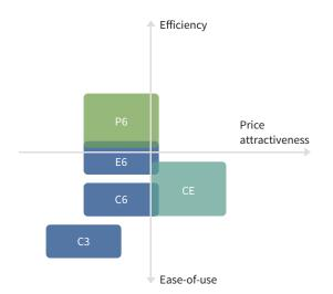
> CoolMOS<sup>™</sup> CE is a general-purpose series, available in 500 V, 600 V, 650 V, 700 V and 800 V, that is optimized for the best balance between cost, efficiency and ease-ofuse. We recommend the CE series as the first choice for cost-sensitive LED lighting applications for diverse topologies.
