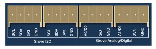
The data wires can be used to drive a variety of Grove-compatible devices, though only those which operate over I<sup>2</sup>C are supported by the impExplorer Kit's two Grove I<sup>2</sup>C headers, both of which connect to the imp001's **hardware.i2c89** bus. The yellow wire provides the clock line; the white wire the data line. Only 3V3 I<sup>2</sup>C devices are supported.
