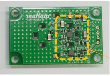
Amplifier and comparator circuits on evaluation board amplifies sensor's output signal and generate digital High/Low signal. (Next page)
