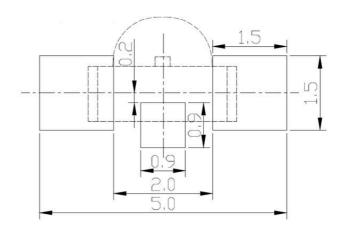
Figure 1. IN-S121AS Solder Pattern
