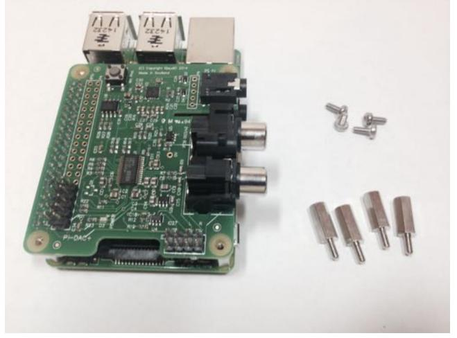
The male/female spacers should replace the 4 screws (these should be retained) previously used to secure the Pi-DAC+ to the Raspberry Pi.
