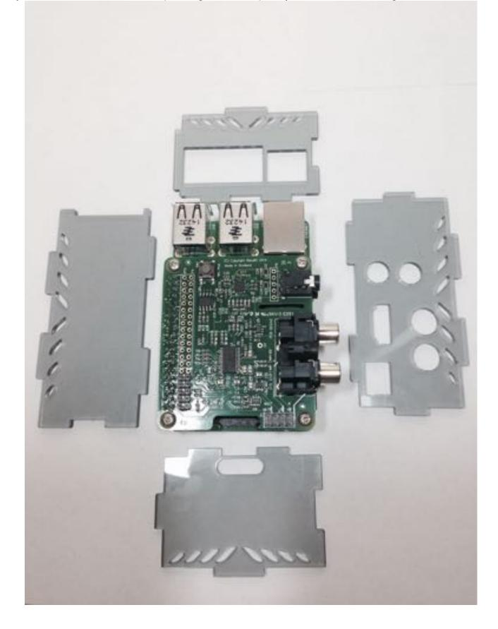
b) Then, build the sides up around the Raspberry Pi. Use sticky tape at each corner to make things simpler to assemble.
