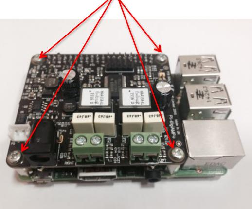
If you are using the Pi-CASE+ then replace the 4x screws beneath the Pi with the 4x 5mm PCB standoffs provided with the Pi-CASE+
