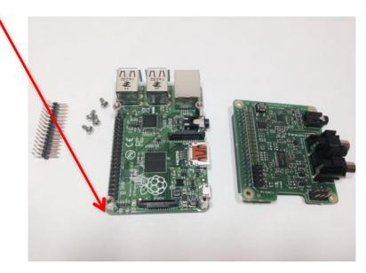
Once the Pi-DAC+ has been fitted the remaining screws can be tightened (finger tight please) as required.
