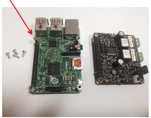
Once the Pi-DigiAMP+ has been fitted the remaining screws can be tightened (finger tight please) as require
