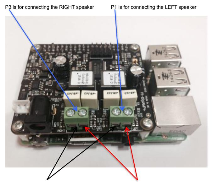
Attach the speaker -ve terminal (often black) to the - on the amplifier output
