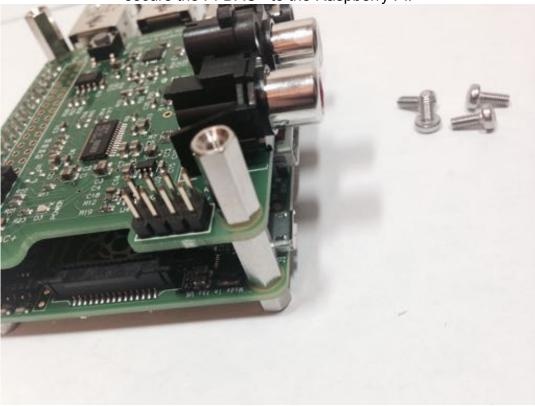
Once the Pi-AMP+ has been fitted the remaining screws (from the Pi-DAC+) can be tightened (finger tight is fine) as required to secure the full PCB stack.
