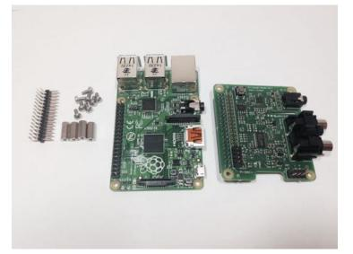
The spacers should be screwed (finger tight only) to the Raspberry Pi before adding the Pi-DAC+.
