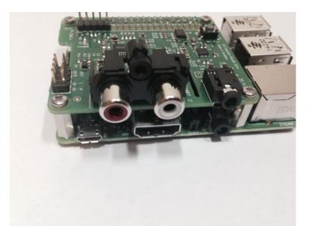
If you are using the Pi-CASE+ then replace the 4x screws beneath the Pi with the 4x 5mm PCB standoffs provided with the Pi-CASE+
