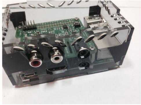
c) Add the base (with text outwards) and screw the case to the Raspberry Pi
