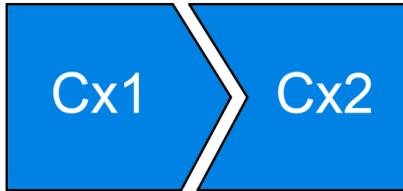
Figure 6.1 : Self Capacitance Swipe Switch Sample Electrodes.
