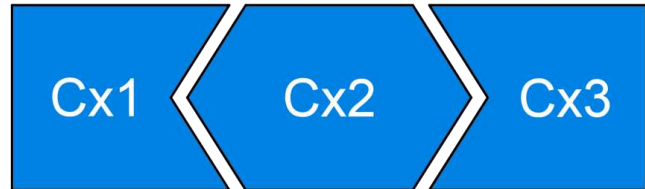
Figure 6.1 : Self Capacitance Swipe Switch Sample Electrodes.
