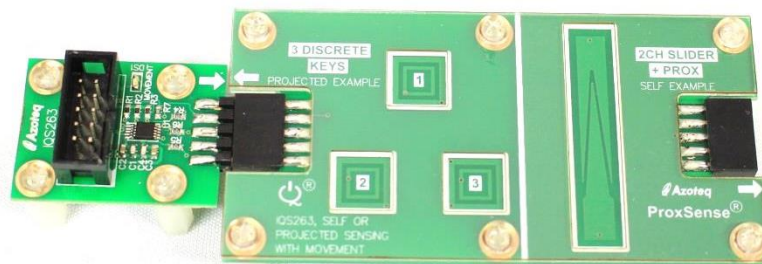
Figure 6.1 3 Keys demo board connected to driver board
