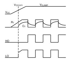
Figure 1. Input/Output Timing Diagram
