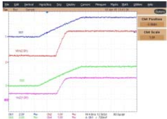
Figure 32 - Prebias Start up Ch1: SS1, Ch2: Vo1, Ch3: SS2, Ch4: Vo2
