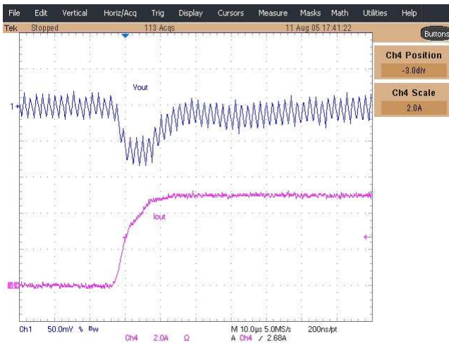
Figure 20 - Load Transient (0-5A) Ch1:Vout, Ch4:Step Load Current
