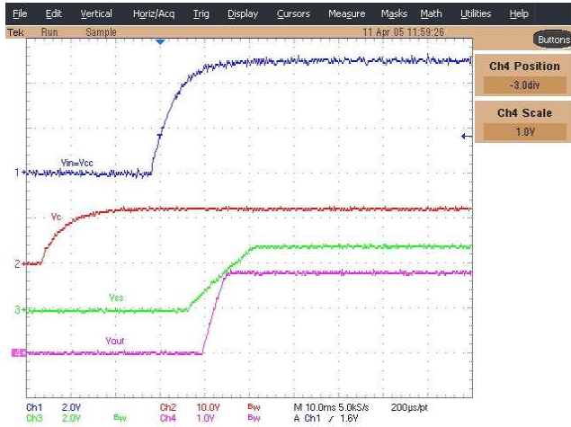
Figure 14 - Start up waveforms Ch1: Vin=Vcc, Ch2: Vc, Ch3: Vss, Ch4: Vout
