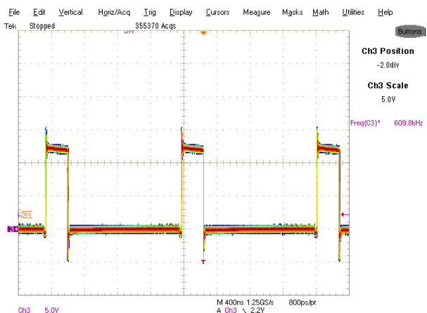
Fig. 21. Inductor node at 6A load Ch 3 :LX
