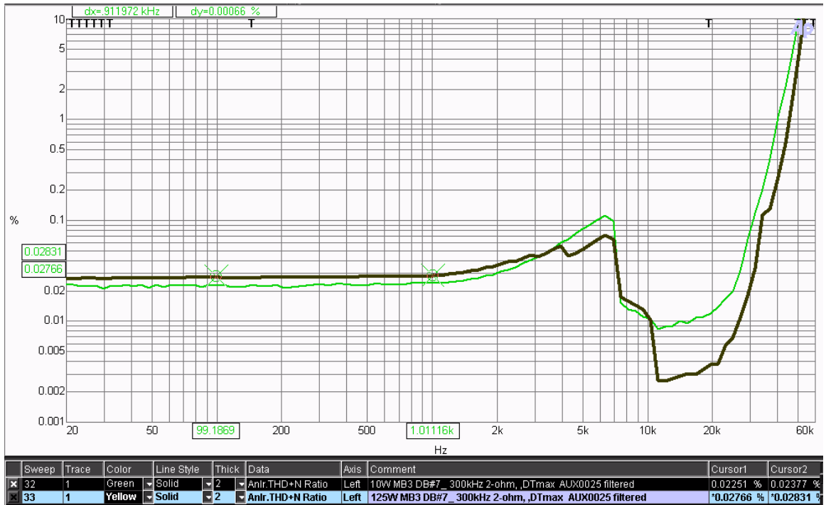
Figure 4 THD+N vs. Frequency at 10W and 125W
