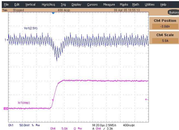
Figure 20 - Load Transient Respons for Vo1 (Io=0 to 10A) Ch1: Vo1, Ch4: Io1
