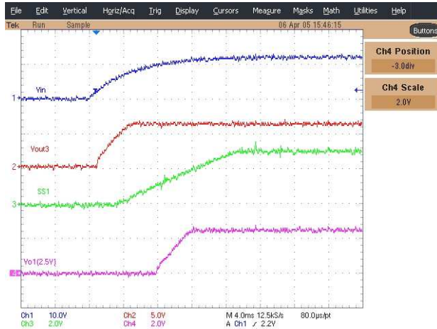
Figure 5 - Start up wavforms for 2.5V output Ch1: Vin, Ch2: Vout3, Ch3: SS1, Ch4:Vo1 (2.5V)
