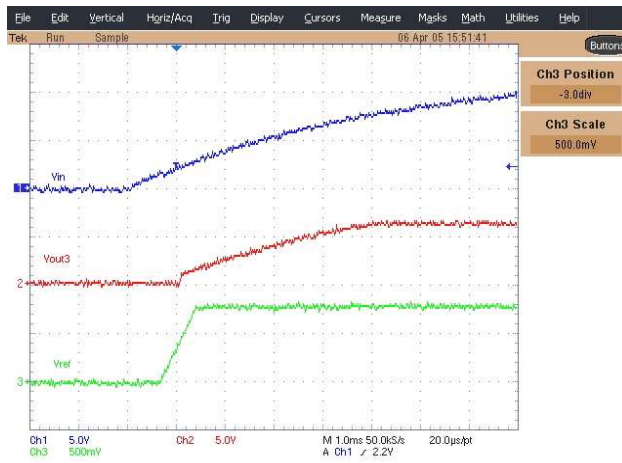
Figure 7 - Start up wavforms Ch1: Vin, Ch2: Vout3, Ch3: Vref
