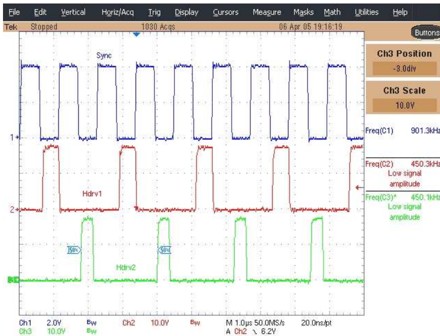
Figure 19 - Extrnal Synchronization Ch1: Extrnal Cloc, Ch2: Hdrv1, Ch3: Hdrv2
