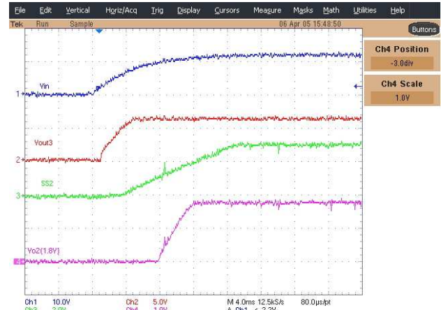
Figure 6 - Start up wavforms for 1.8V output Ch1: Vin, Ch2: Vout3, Ch3: SS2, Ch4:Vo2 (1.8V)
