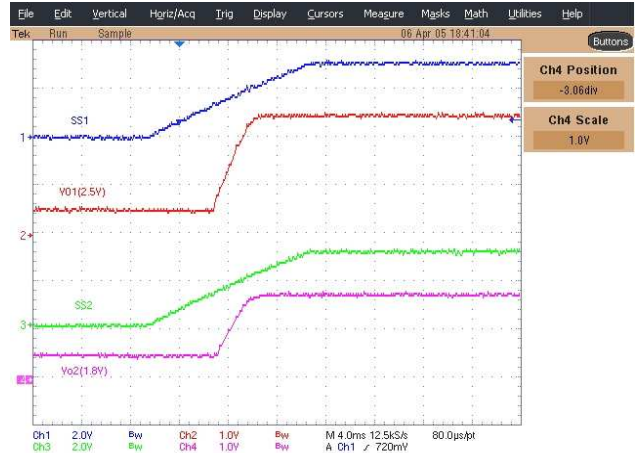
Figure 16 - Prebias Start up Ch1: SS1, Ch2: Vo1, Ch3: SS2, Ch4: Vo2
