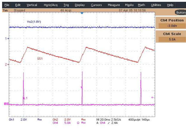
Figure 15 - 2.5V output shorted Ch1: Vo2, Ch2: SS1, Ch3: Inductor Current
