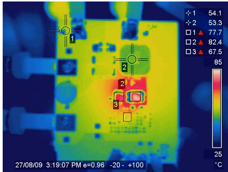
Figure 19: Thermal Image @19Vin, 24A, With CP On
