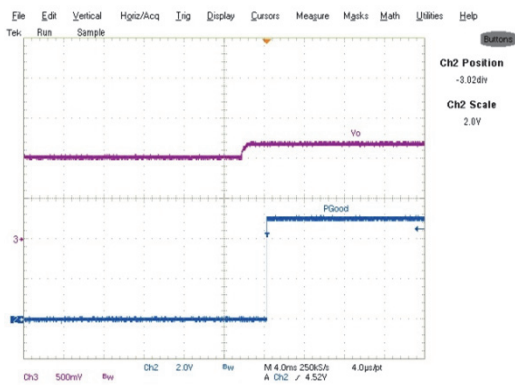
Fig. 9: Start up with 1V Pre Bias, 0A Load, Ch 2 :P Good , Ch 3 :V o
