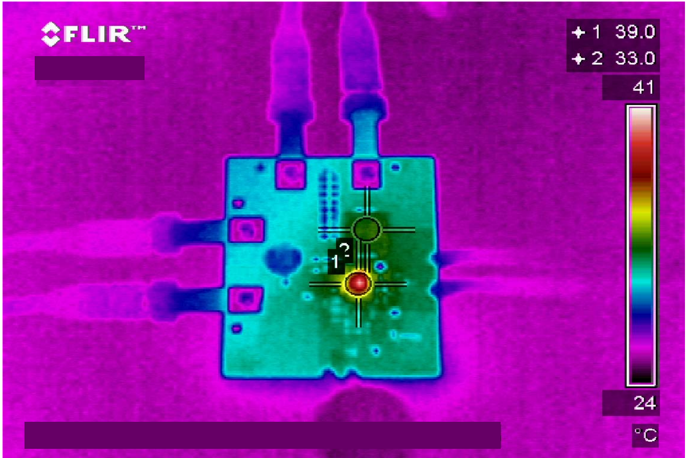
Fig. 17: Thermal Image at 4A load Test points 1 and 2 are IR3842 and inductor, respectively.
