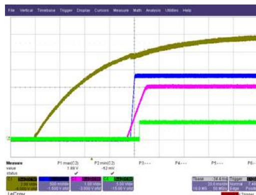
Fig. 8. Start up at 6A Load, Ch 1 :V in , Ch 2 :V o , Ch 3 :V ss , Ch 4 :V PGood
