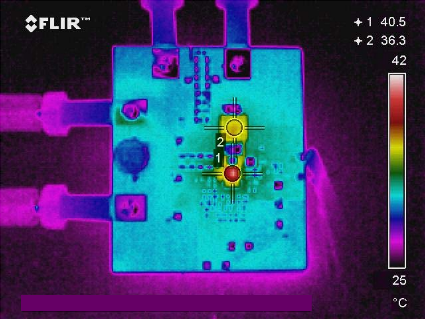
Fig. 18: Thermal Image at 4A load Test points 1 and 2 are IR3853 and inductor, respectively.
