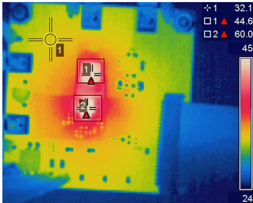
Fig. 17: Thermal Image (IR3863: 60°C, Inductor: 45°C, PCB: 32°C)
