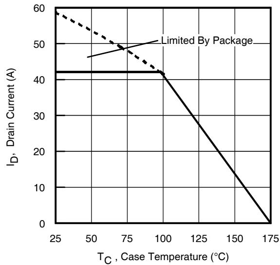
**Fig 9.** Maximum Drain Current vs.
