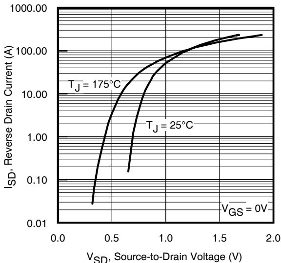
**Fig 7.** Typical Source-Drain Diode
