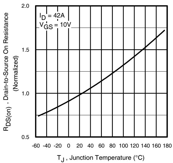
**Fig 4.** Normalized On-Resistance
