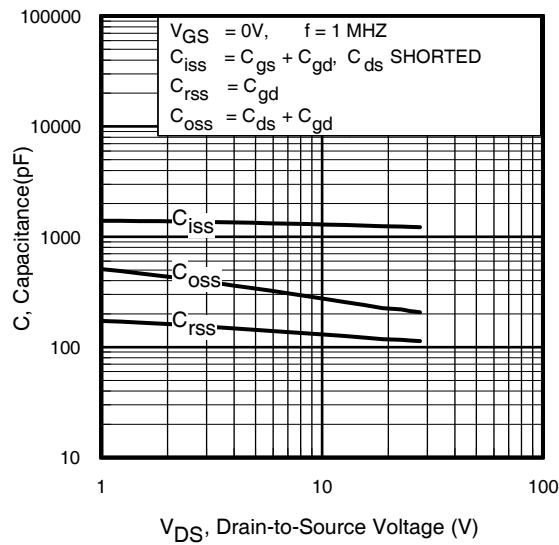
**Fig 5.** Typical Capacitance vs.
