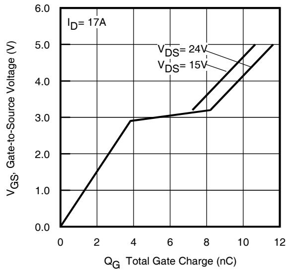
**Fig 6.** Typical Gate Charge vs.
