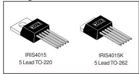
The IRIS4015(K) is a dual mode voltage and current controller combined with a MOSFET in a single package. The IRIS4015(K) is designed for use in AC/DC switching power supplies up to 230VAC nominal input, and is capable of 180W for a universal line input. The device operates on a quasi-resonant or Pulse Ratio Control (PRC) basis, and thereby variable frequency operation.
