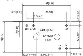
Case No.IRM03 Unit:mm[inch] Tolerance:±0.5[±0.02] unless otherwise specified
