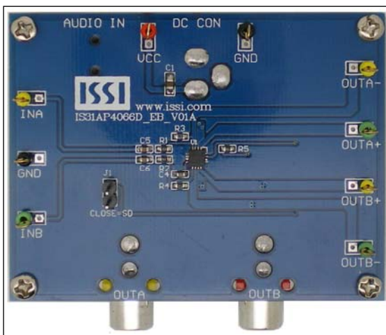
Figure 1: Photo of IS31AP4066D Evaluation Board
