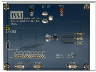
Figure 1: Photo of IS31BL3212 Evaluation Board
