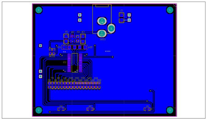
Figure 6: Board PCB Layout-Bottom Layer
