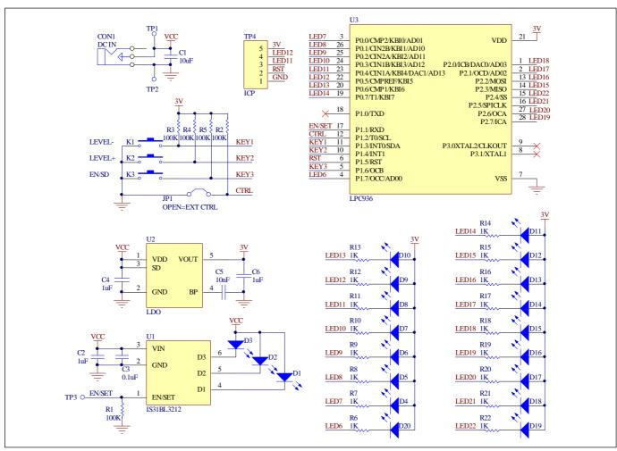
Figure 2: IS31BL3212 Application Schematic
