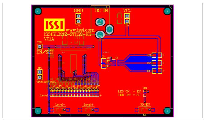
Figure 4: Board PCB Layout- Top Layer
