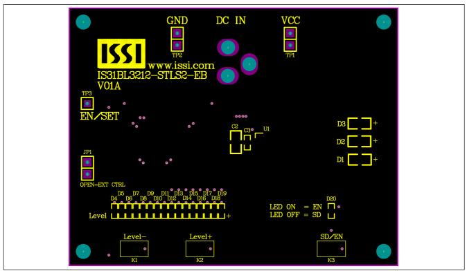
Figure 3: Board Component Placement Guide -Top Layer
