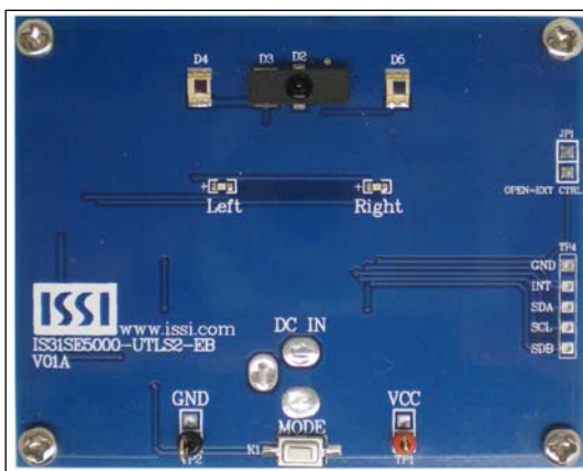
Figure 1: Photo of IS31SE5000 Evaluation Board
